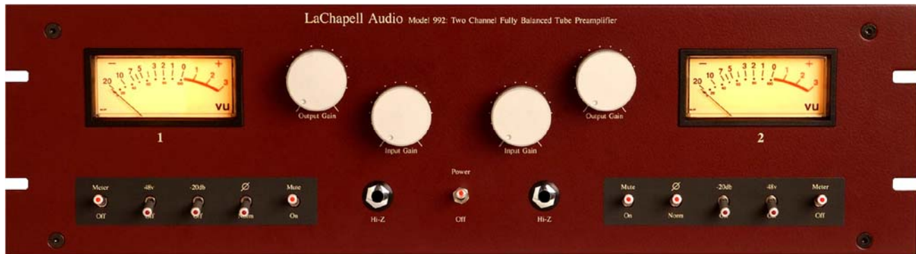
FIGURE 2.1 the five LED tipped toggles on channel 1 are (from left to right) Meter, 48v, -20db, Polarity Reverse and Mute. The two lower knobs on the inside are for input gain and the two upper knobs are for output gain.
